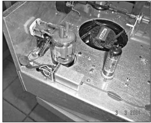
Fig 7.5: Close-up view of the 6m output network in the dual-band amplifier
