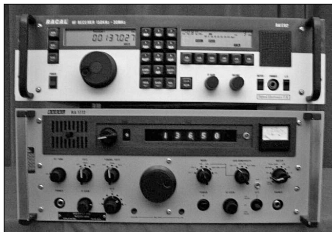
Fig 10.2: Racal RA1792 (top), and RA1772 perform well on LF
