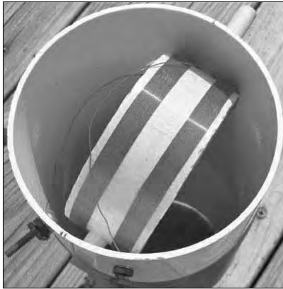
Fig 72: A home-made variometer
