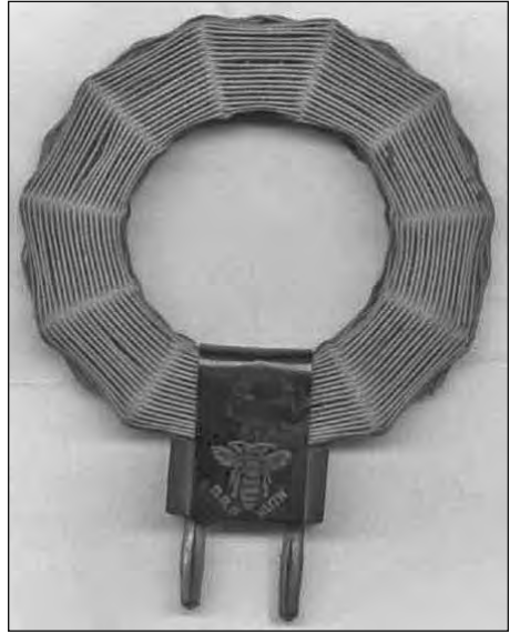
Fig 74: A plug-in honeycomb coil
