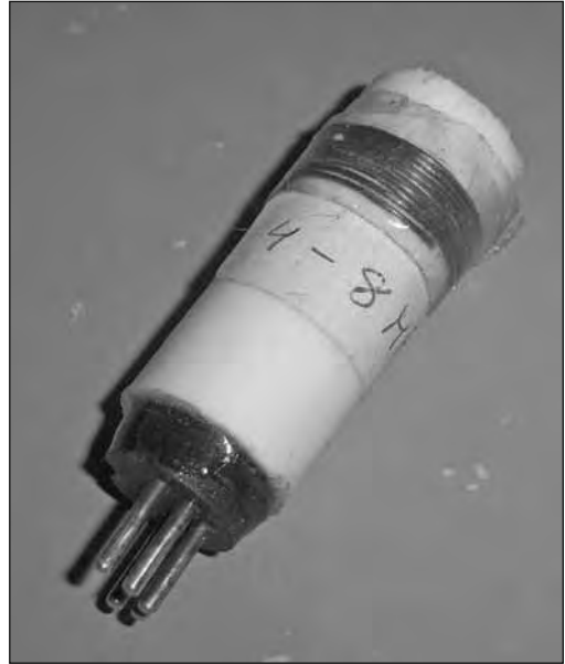
Fig 71: Plug-in cylindrical coil
